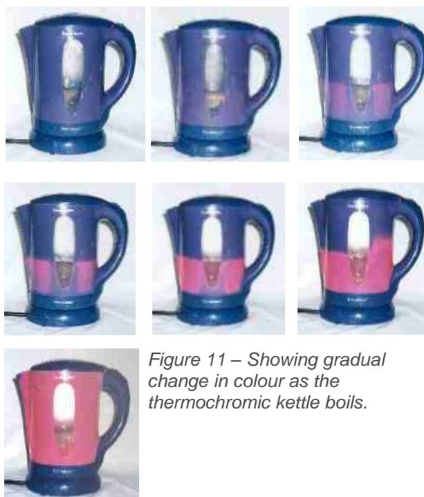
Figure 11 – Showing gradual change in colour as the thermochromic kettle boils.
