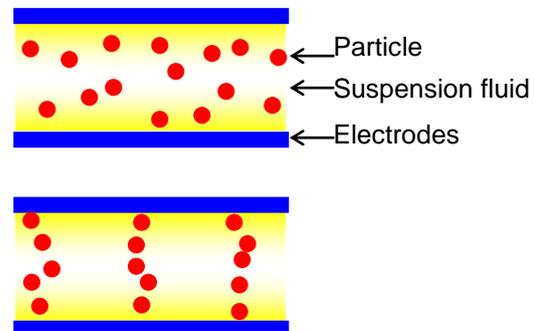
Figure 7 – Schematic diagram showing the structure of a electrorheological fluid between two electrodes. The top figure shows the structure in a low field strength where the particles are randomly distributed. When a higher field strength is applied, as in the bottom diagram, the particles align causing a change in the viscosity of the fluid.
