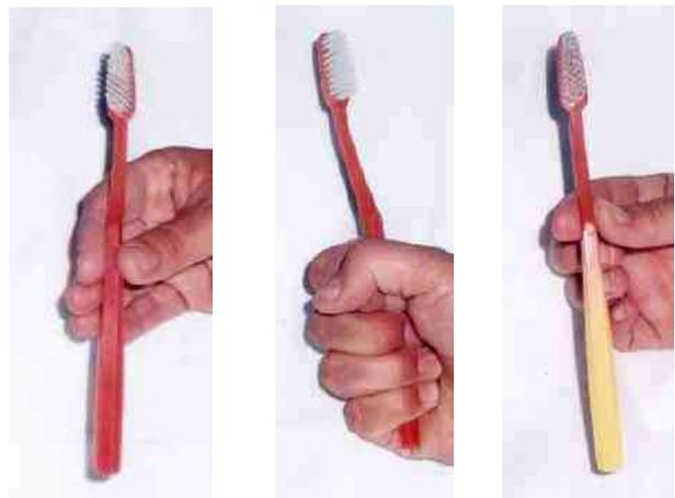
*Figure 10 – A thermochromic toothbrush at room temperature, being warmed by holding in the hand and when warm.*
