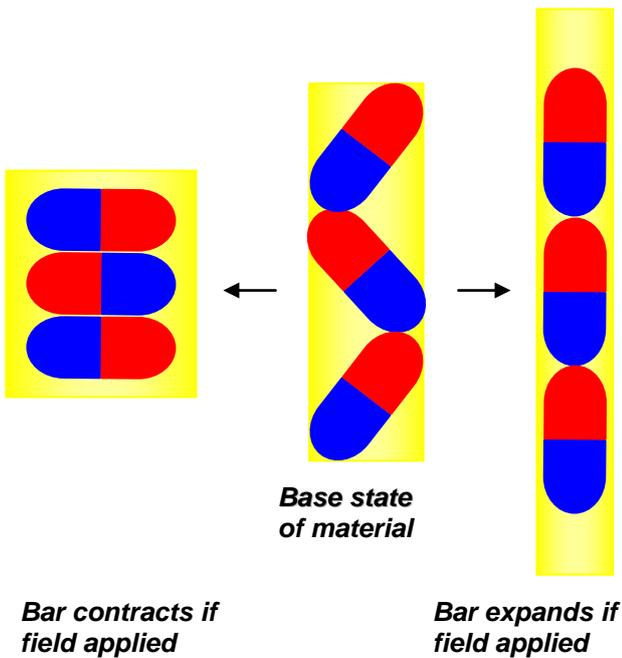
*Figure 6 – Magnetostrictive materials are made up from domains (represented by red and blue bar magnets). If a magnetic field is applied the bar either decreases in length from its base state (centre to left) or increases in length (centre to right) depending on the polarisation of the applied field.*
