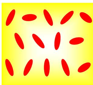
Figure 9 – A liquid crystal contains needle shaped particles which are arranged randomly below the transformation temperature (top). Above this temperature the particles are aligned, changing how the material reflects light, thus showing a change in colour (bottom)
