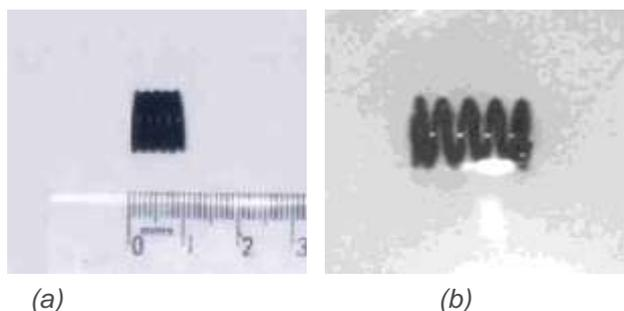
Figure 5 – Showing the two memory shapes of a memory metal wire coil or 'spring'. In (a) the spring is at room temperature and in (b) the higher temperature state has been activated by pouring on boiling water.
