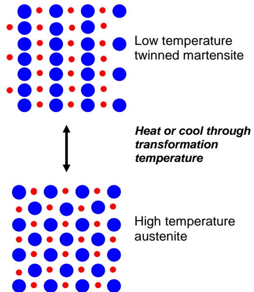
Figure 1 – Change in structure associated with the shape memory effect.
