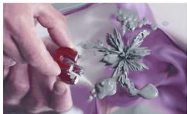
Figure 8 - A puddle of magnetorheological fluid stiffens in the presence of a magnetic field. (courtesy of Sandy Hill / University of Rochester)
