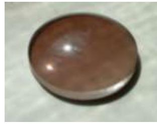
*Figure 13 – An unground, photochromic spectacle lens sat on a sunny windowsill.*
